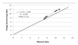
**Fig. 3.** The relationship between the length values of three rice varieties obtained by image processing method and manual procedure at different processing levels.
